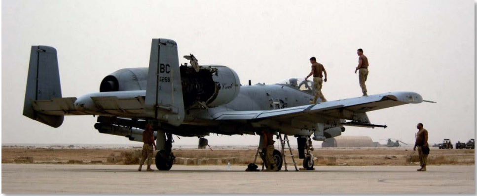
Şekil 29. A-10 Thunderbolt II maintenance members inspect aircraft after it was hit by an Iraqi missile
