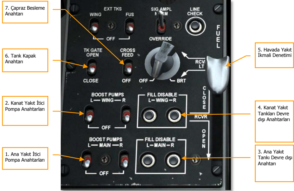
Şekil 298. Fuel System Panel
