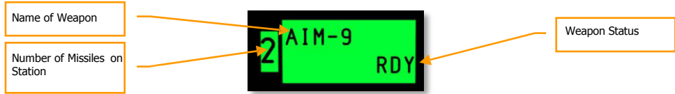
Şekil 466. AIM-9 Station Box Loading
